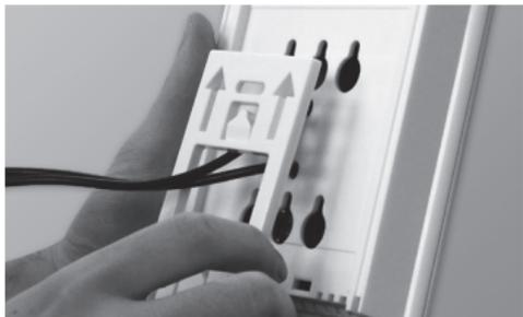
Then, remove the mounting base at the back of the thermostat by tilting it downward, then towards you.
